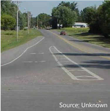
An offset right-turn lane can help improve poor sight distance for drivers stopped on the minor road approach.
