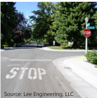
Source: Lee Engineering, LLC The STOP pavement marking along this approach adds emphasis to the stop condition.
