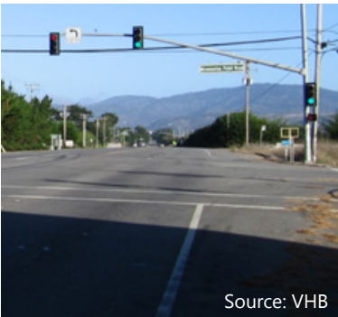
This traffic signal offers a protected phase for left turns from the major road.
